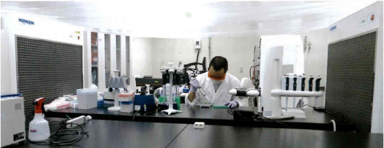
(Pic.1) A pair of units of the KOACH are placed across the table on the left and right. Purified airflows blown by these units keep the work area at high level of cleanliness all times.
